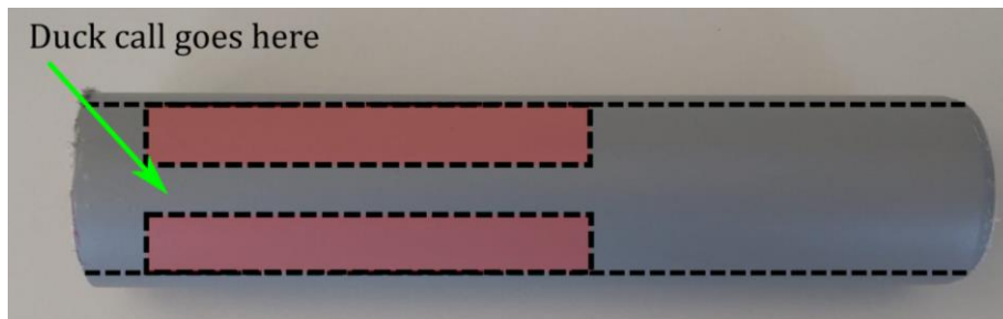
Figure 5.3.3. An assembled vowel resonator.
